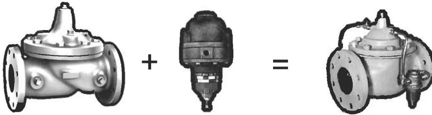
When there is no pressure on the assembly, the spring and the weight of the assembly hold the valve closed. When placed in-line and pressure is applied, the valve opens. If inlet pressure is piped into the cover chamber the valve closes tightly.
