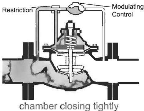
**Modulating valves** open and close based on pressure, like non-throttling valves. Modulating valves provide the following operations:
